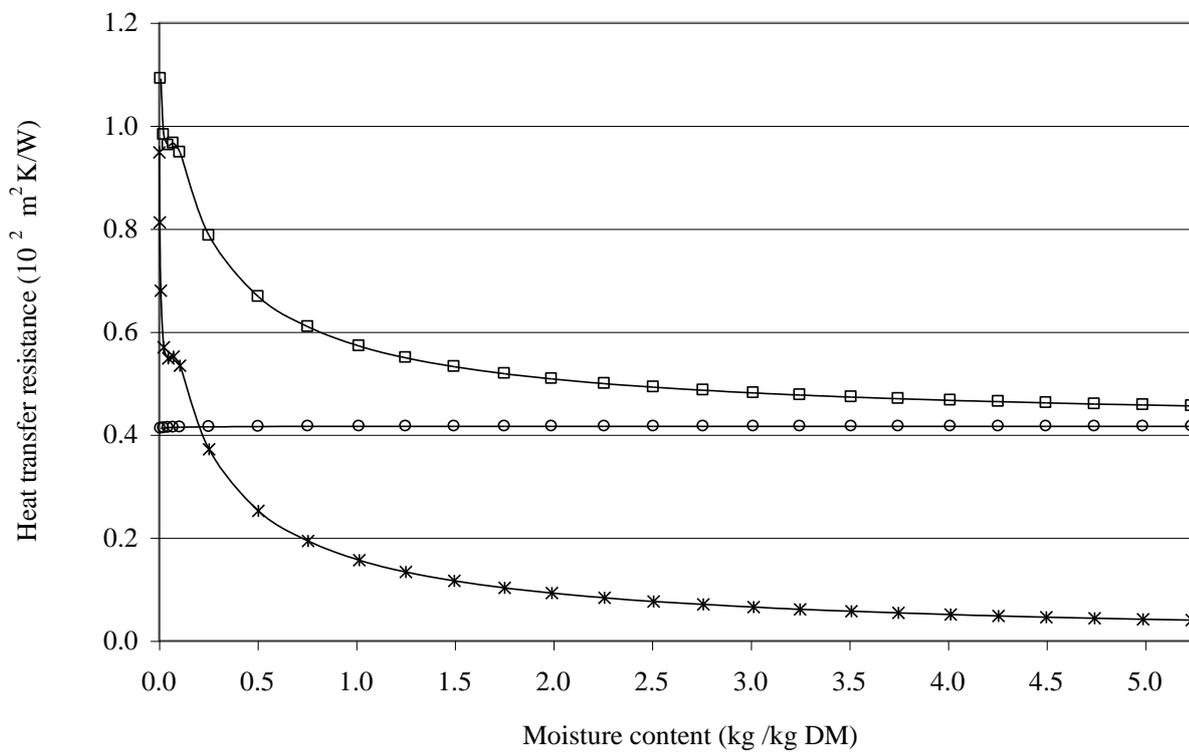
Figure 14 – Measured (dot) and adjusted (line) drying kinetics of the digested sewage sludge coming from Albi City for (□)  $T_{\text{wall}} = 160^{\circ}\text{C}$  and (○)  $T_{\text{wall}} = 120^{\circ}\text{C}$  ( $\omega = 40$  rpm,  $d = 1.15 \cdot 10^{-3}$  m).
