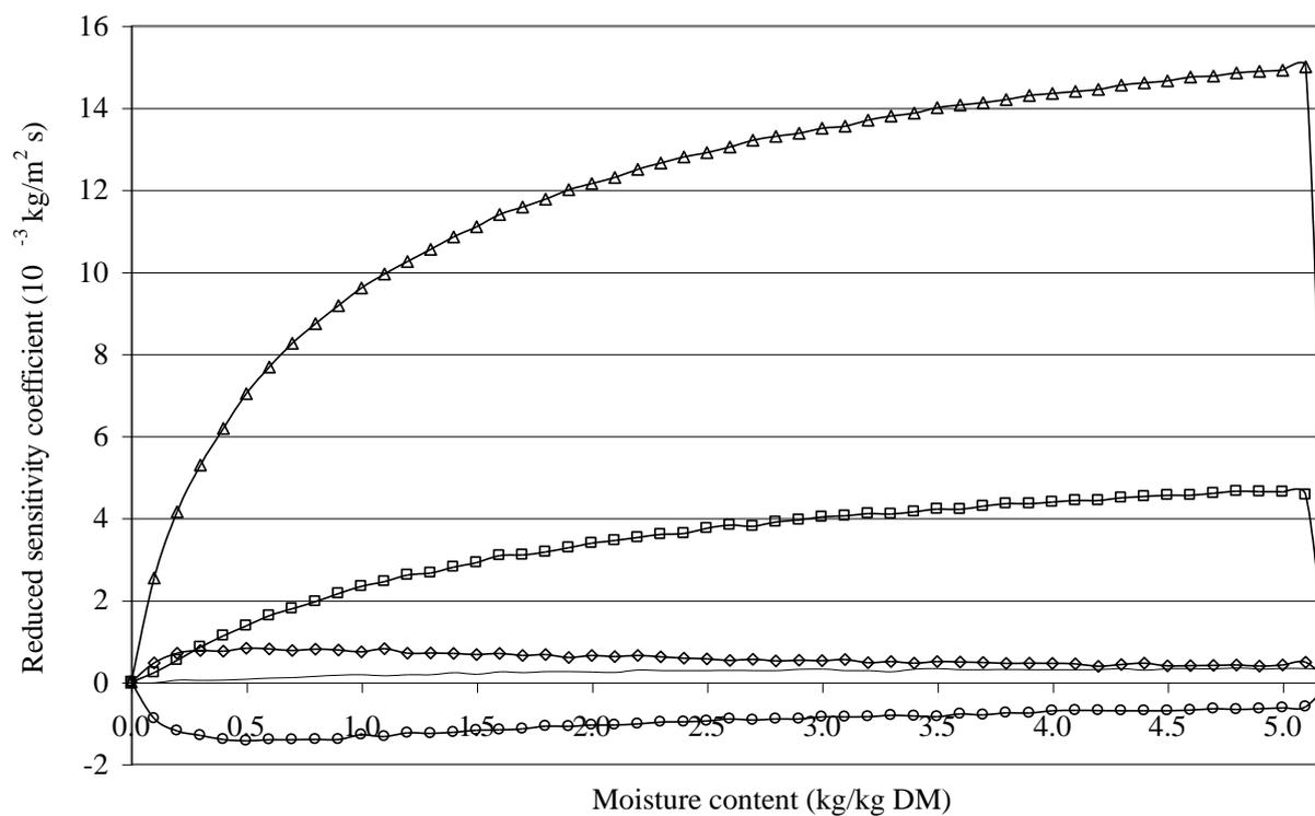
Figure 4 – Reduced sensitivity coefficients to parameters connected with product properties : (—+—) particle diameter, (—○—) particle rugosity, (—□—) thermal conductivity,(—△—) specific heat and (—) apparent density.
