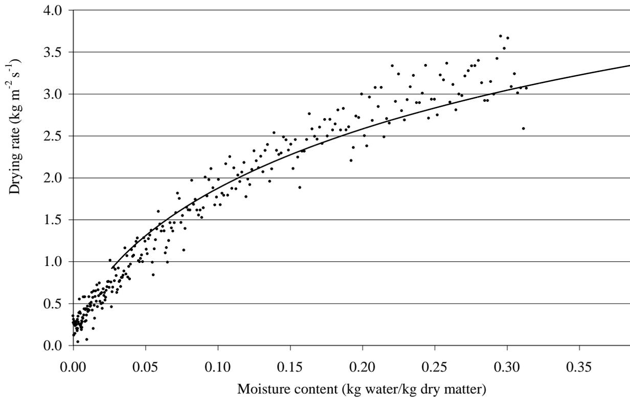
Figure 11 – Measured (—) and adjusted (—□—) drying kinetics of the digested sewage sludge coming from Albi City ( $T_{\text{wall}} = 180^{\circ}\text{C}$ ,  $\omega = 40 \text{ rpm}$ ,  $d = 1.15 \cdot 10^{-3} \text{ m}$ ).
