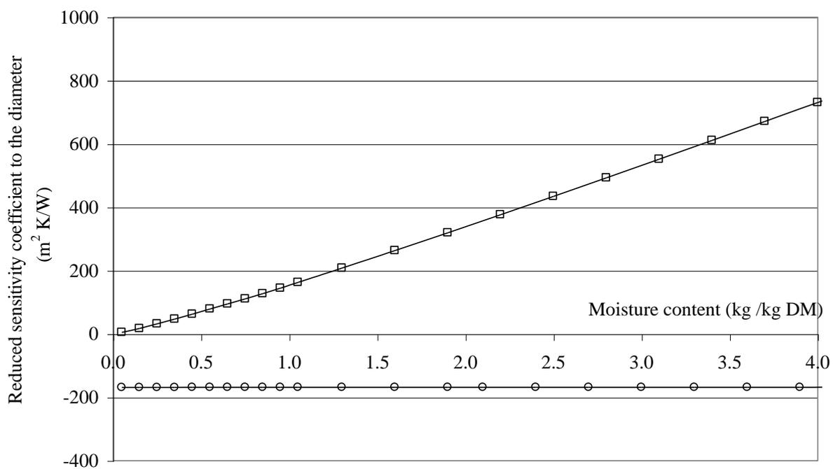
Figure 8 – Reduced sensitivity coefficients of the contact resistance to the stirrer speed and the moisture content for  $10^{-3}$  m activated alumina balls.
