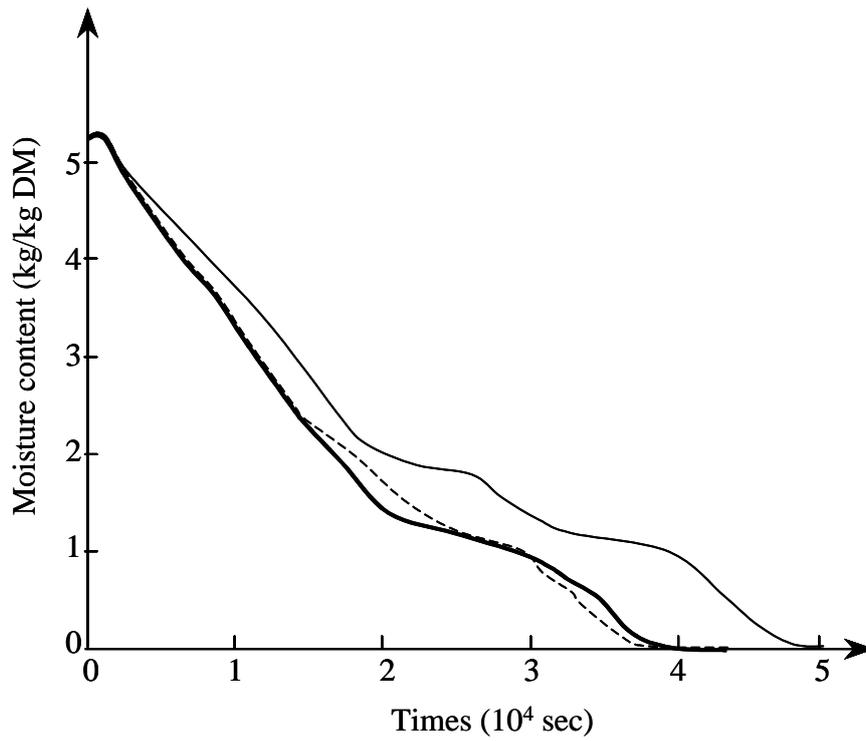
Figure 16 Measured (dot) and adjusted (line) drying kinetics of an anaerobically digested sludge ( (+),  $d=1.15 \cdot 10^{-3}$  m) and an extended aeration one (  $\circ$ ),  $d=0.9 \cdot 10^{-3}$  m) for  $T_{\text{wall}} = 160^\circ\text{C}$  and  $\omega = 40$  rpm.
