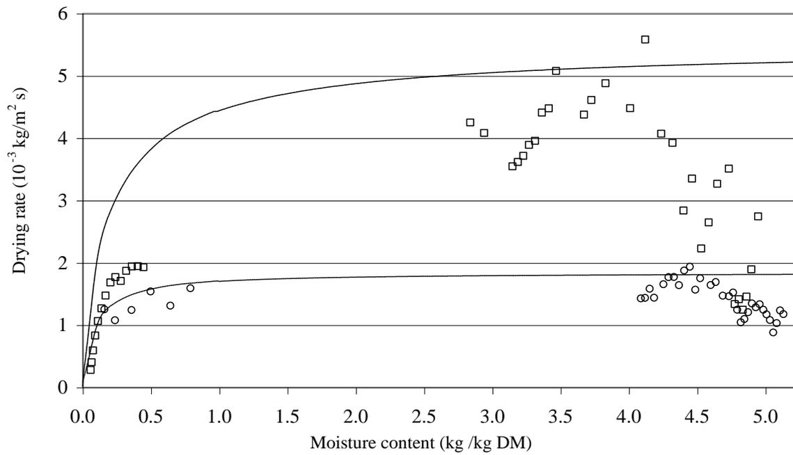
Figure 15 – Influence of the stirrer speed, (+)  $\omega = 20$  rpm, (o)  $\omega = 40$  rpm and (--)  $\omega = 60$  rpm, on the experimental drying kinetic ( $T_{\text{wall}} = 120^\circ\text{C}$ ).
