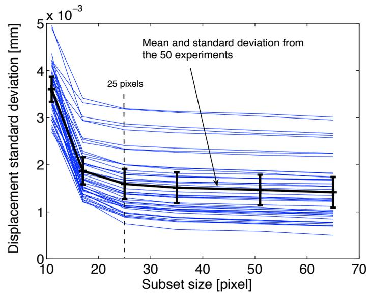
Figure 6:  $\sigma(U)$  versus the subset size for 50 imposed solid body displacements of the bending test castable specimen. In large line, the mean value and the standard deviation (error bars) of  $\sigma(U)$  for all the experiments are plotted.
