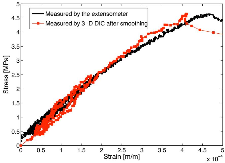
Figure 13: Comparison of behavior curves obtained by 3-D DIC and by an extensometer during a tensile test performed on a FRRC fired at 500°C.
