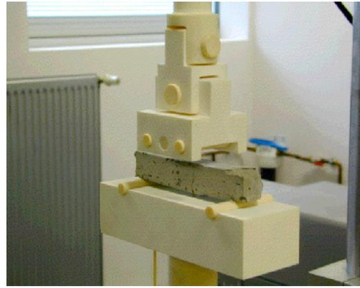
Figure 11: Zoom on the active parts of the tensile test device (left) and of the 4-point bending test device (right) in the room temperature configuration.
