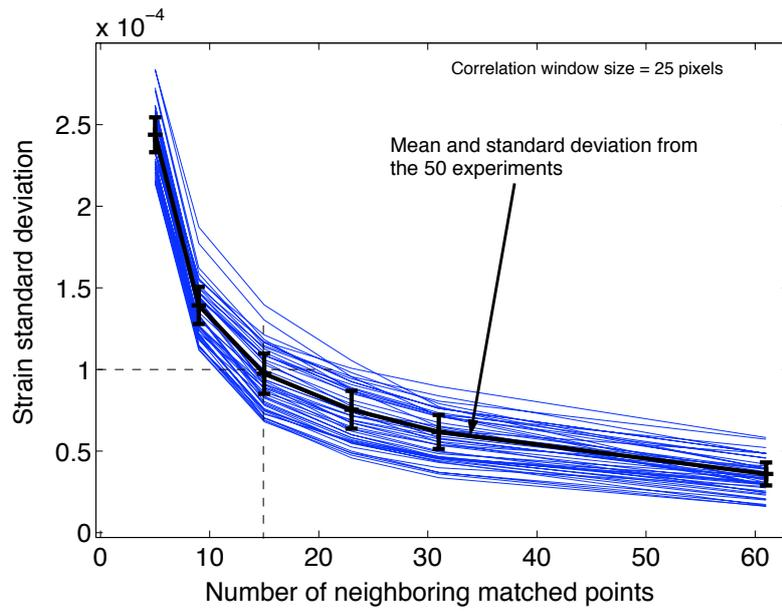
Figure 9:  $\sigma(\varepsilon)$  versus the nmp parameter (or optical gauge length) for 50 experiments. As a large line the mean value and the standard deviation (error bars) of  $\sigma(\varepsilon)$  for all the experiments are plotted.
